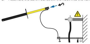
3. Contact the test object with the tip of the earth rod.
