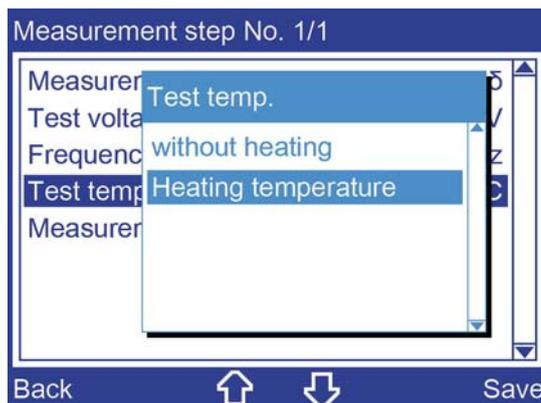
3. Select "Heating temperature" by pressing the arrow keys.
