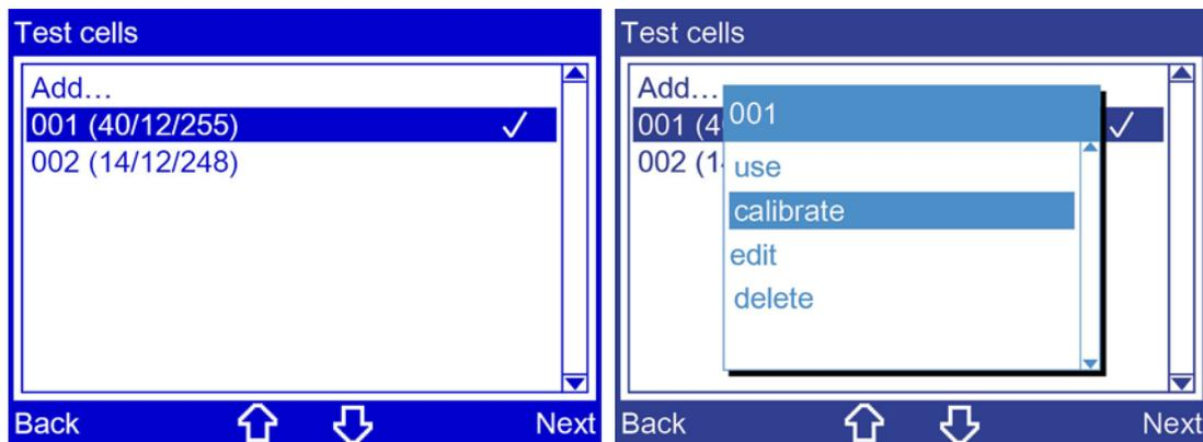
3. Select a test cell using the arrow keys.
