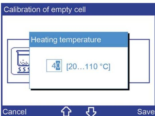
9. Select the heating temperature for the empty cell calibration using the number keys on the membrane keypad.
