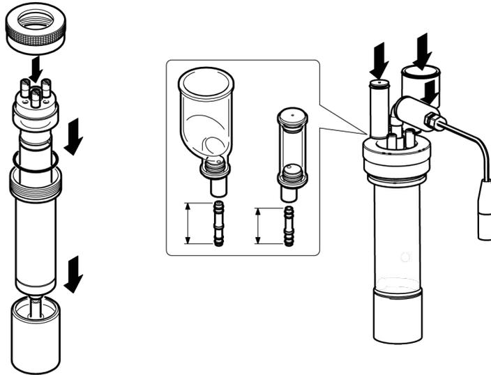
4. Place the high voltage electrode on the base.
