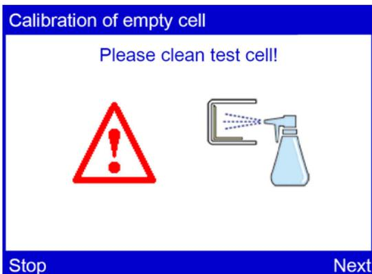
7. Clean the test cell if it has not yet been cleaned. (see "Clean the test cell" on page 19)
