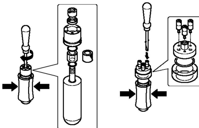
1. Mount the individual parts and tighten the slotted nuts properly.
