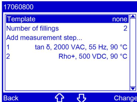
You can view and edit all the parameters of a measurement and define a new user-defined measurement in this menu.
