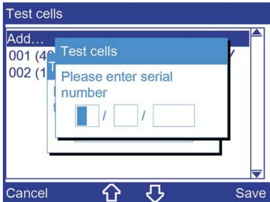
7. The serial number is on the side of the test cell. Enter the serial number with the number keys on the membrane keypad.
