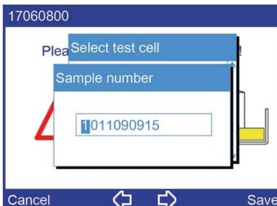
17. If you want to expand the suggested sample number, do so or enter any sample number with the number keys on the membrane keypad.
