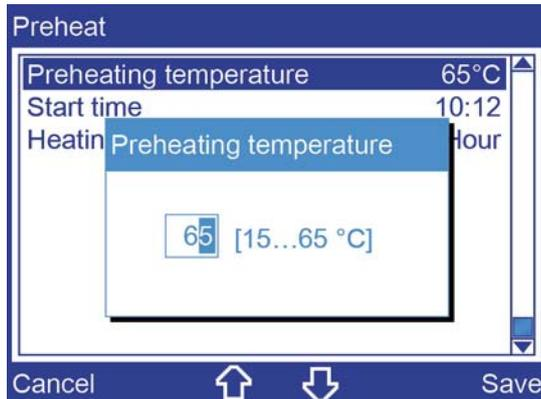
7. Select the preheating temperature with the number keys on the membrane keypad.
