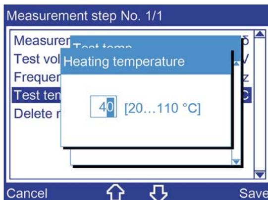
5. Select the heating temperature with the number keys on the membrane keypad.
