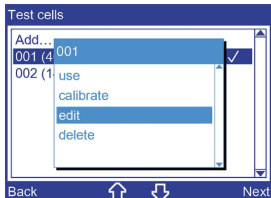
3. Select a test cell using the arrow keys.
