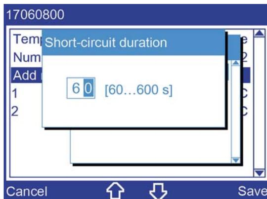
Select the short-circuit duration by pressing the arrow keys or the number keys on the membrane keypad and confirm with “Save”.
