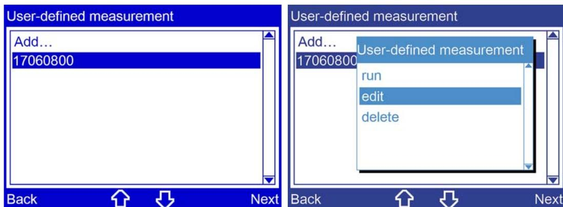
1. Select a saved measurement by pressing the arrow keys.
