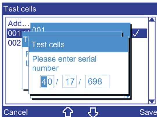
9. If you want to change the serial number, enter another serial number with the number keys on the membrane keypad. The serial number is on the side of the test cell.
