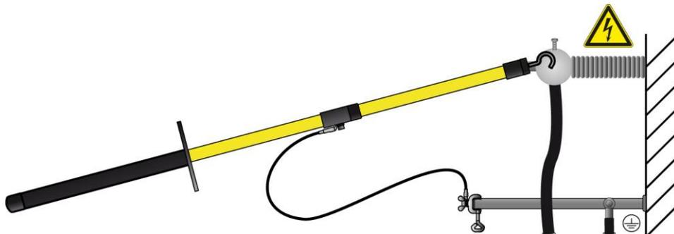
4. Observe the minimum discharge period in accordance with the capacity of the test object.
