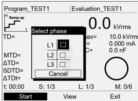
If the function **Split MWT measurement** is activated, the context menu is used additionally for selecting the measurement stage (Ramp-up or MWT) on the respective phase. The phases on which the respective measurement stage has already been carried out are indicated by means of a tick. If a measurement stage on a phase was cancelled, this is indicated by a cross.
