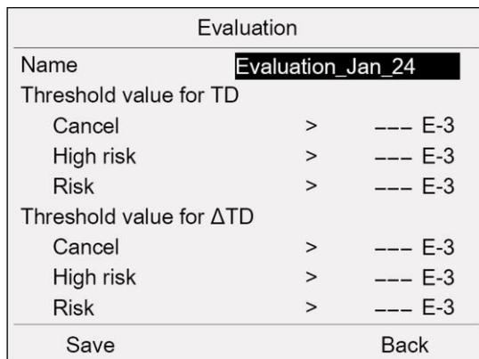
2. If you wish to assign a different name, select the input field **Name** and press the rotary knob to confirm.
