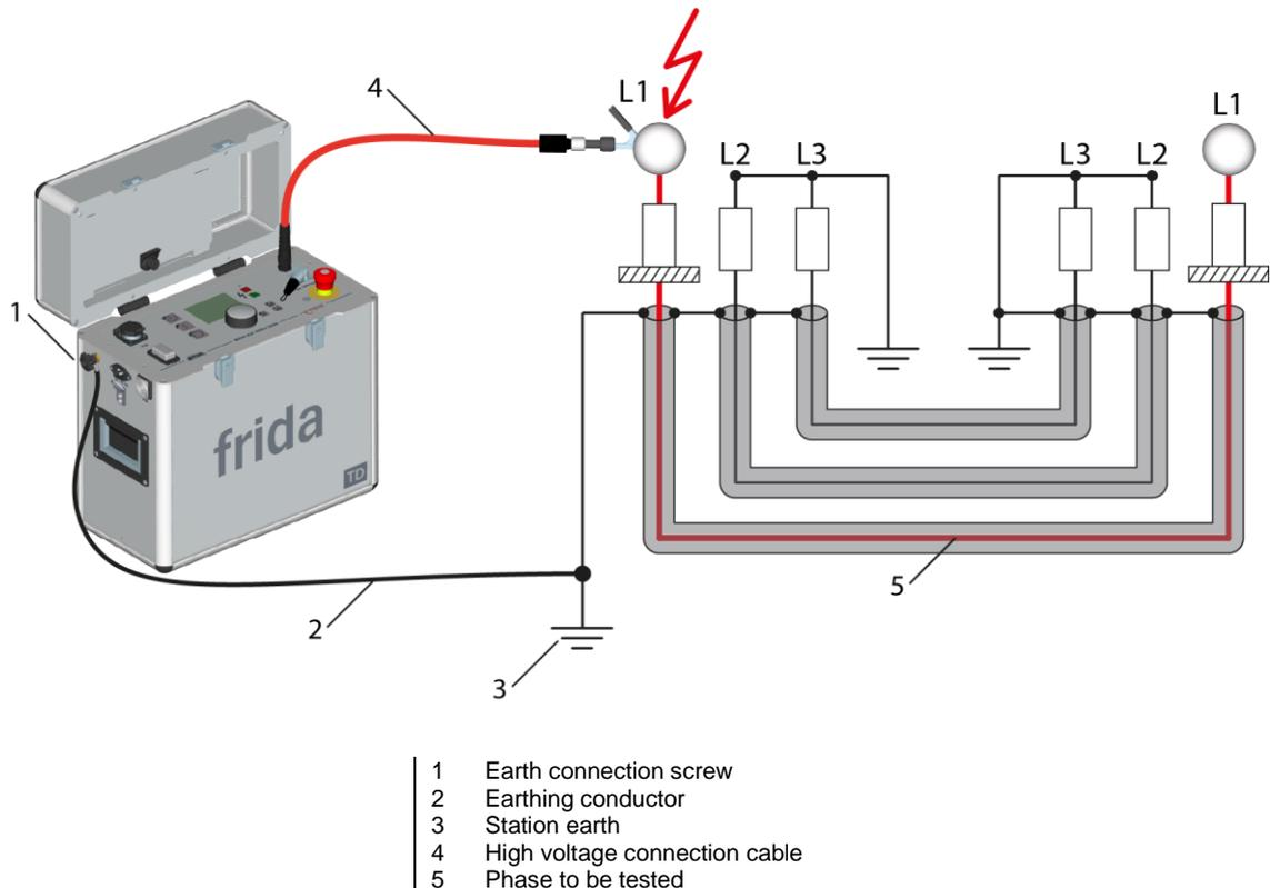
1. The scope of delivery of frida TD comprises an earthing conductor. Connect the earthing conductor to the station earth.
