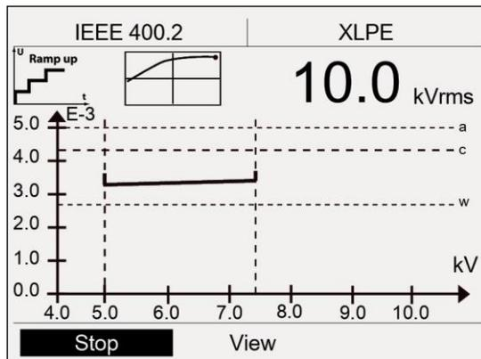
**Diagram tan δ versus time (for the MWT stage)**
