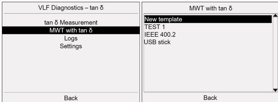
3. In the menu **MWT with tan  $\delta$**  select the menu item **New template** and press the rotary knob to confirm.
