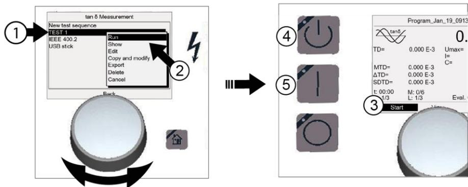
**Dissipation factor measurement process:**
