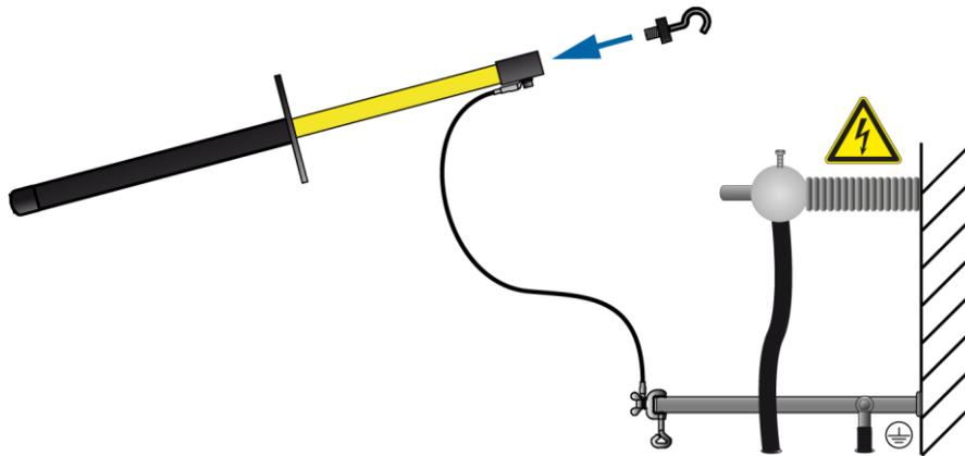
3. Contact the test object with the tip of the earthing rod.
